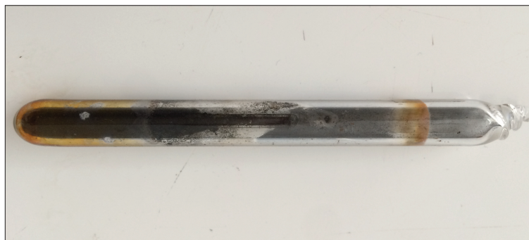
Figure 6.3: Photograph of reaction tube after heat treatment, condensed Rb is observed as an orange hue implying a failed reaction
