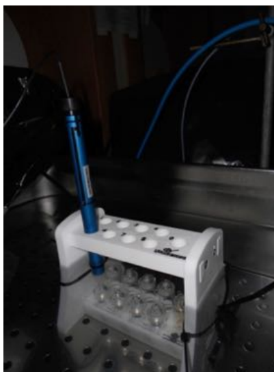
Figure 3.3: Unisense micro-respiration system setup for oxygen uptake of particles in a water bath.
