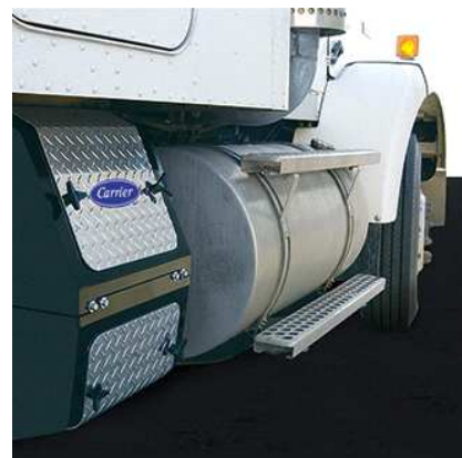
(b) Auxiliary Power Unit
