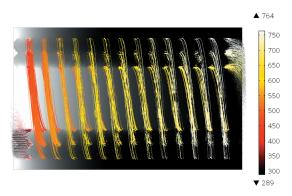
Figure 15. Detail on the T50 heat exchanger meshed domain
