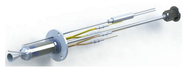
Figure 3. Assembly view with transparent thruster housing showing coaxial heating elements
