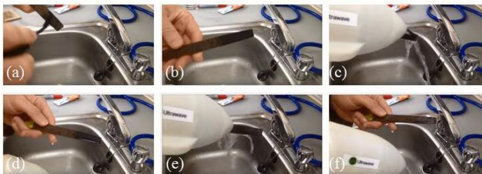
Figure 7. Cleaning a workbench file using UAS. (a,b) A workbench file has mascara make-up smeared onto it. (c) A StarStream device – with the ultrasound turned off - passes a stream of cold water with no additives over this contaminant, and afterwards (d) there has been no observable cleaning. However, when (e) the same water stream has ultrasound added to it, then afterwards (f) both the contaminant has been removed. The panels are stills from the video available at: https://www.youtube.com/watch?v=22tUGEGyk10
