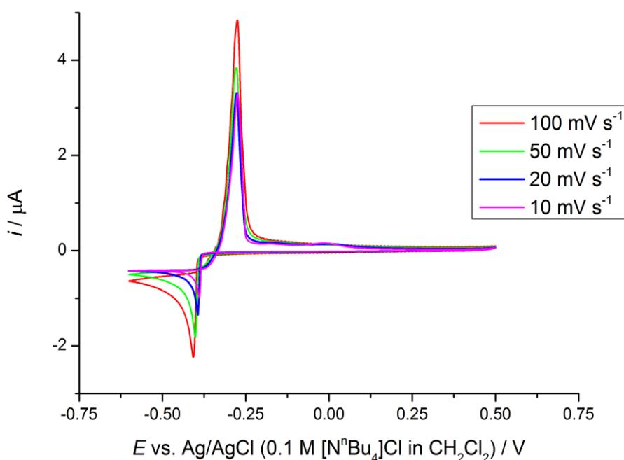
**Figure 2** Cyclic voltammograms of 0.5 mM [PPh<sub>4</sub>][PbCl<sub>3</sub>] in CH<sub>2</sub>Cl<sub>2</sub> as a function of scan rate, recorded at a 0.5 mm diameter Pt disk. The supporting electrolyte used was 100 mM [PPh<sub>4</sub>]Cl.
