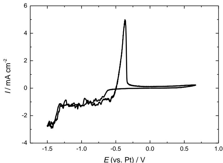
**Figure 5** Cyclic voltammetry of 2 mM [PPh<sub>4</sub>][PbCl<sub>3</sub>] + 50 mM [N<sup>n</sup>Bu<sub>4</sub>]Cl at a Pt disk electrode (surface area 1.963 x 10<sup>-3</sup> cm<sup>2</sup>) in scCH<sub>2</sub>F<sub>2</sub> (17.5 MPa, 360 K). The potential scan rate was 50 mV s<sup>-1</sup>.
