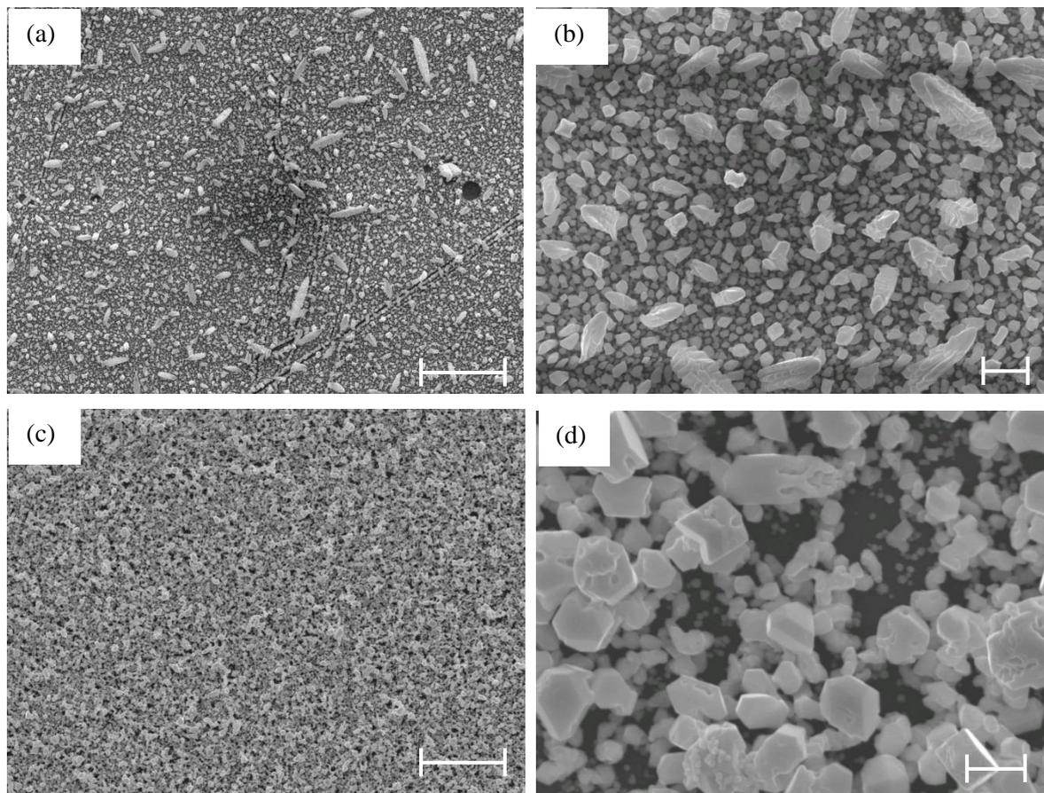
**Figure 6** SEM micrographs of Pb electrodeposited on planar electrodes in  $\text{CH}_2\text{Cl}_2$ . The substrates and magnifications used are (a) Au, x2000 (scale bar = 10  $\mu\text{m}$ ), (b) Au, x10000 (scale bar = 1  $\mu\text{m}$ ), (c) TiN, x2000 (scale bar = 10  $\mu\text{m}$ ), (d) TiN, x13000 (scale bar = 1  $\mu\text{m}$ ).
