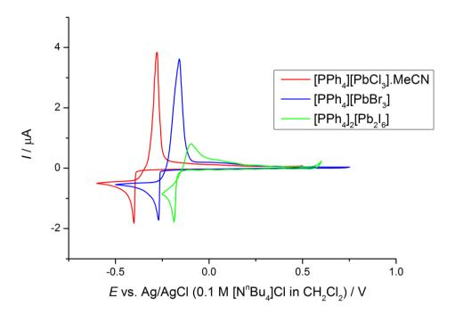
**Figure 4** Cyclic voltammograms of [PPh<sub>4</sub>][PbX<sub>3</sub>] (X = Cl, Br, I) in  $CH_2Cl_2$  recorded at a 0.5 mm diameter Pt disk. The composition of each electrolyte system was 0.5 mM (based on Pb content) of (i) [PPh<sub>4</sub>][PbCl<sub>3</sub>], (ii) [PPh<sub>4</sub>][PbBr<sub>3</sub>] and (iii) [PPh<sub>4</sub>]<sub>2</sub>[Pb<sub>2</sub>I<sub>6</sub>] with 100 mM [PPh<sub>4</sub>]X. The potential scan rate was 50 mV s<sup>-1</sup>.
