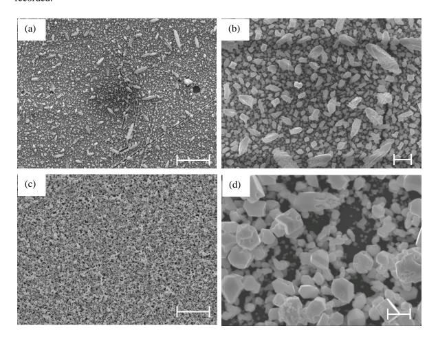
**Figure 6** SEM micrographs of Pb electrodeposited on planar electrodes in  $CH_2Cl_2$ . The substrates and magnifications used are (a) Au, x2000 (scale bar = 10  $\mu$ m), (b) Au, x10000 (scale bar = 1  $\mu$ m), (c) TiN, x2000 (scale bar = 10  $\mu$ m), (d) TiN, x13000 (scale bar = 1  $\mu$ m).
