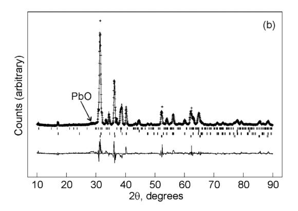
**Figure 7** Rietveld fits to the GIXRD patterns of Pb films deposited on (a) TiN or (b) gold. In each plot the crosses mark data points, the top continuous line the fit, tick marks the allowed reflection positions and the bottom continuous line the difference. In (a) the upper tick marks are for PbO and the lower for Pb; in (b) the sequence is AuPb<sub>3</sub> (top), Au, AuPb<sub>2</sub>, Pb (bottom). Peaks due to phases not included in the fit are marked.
