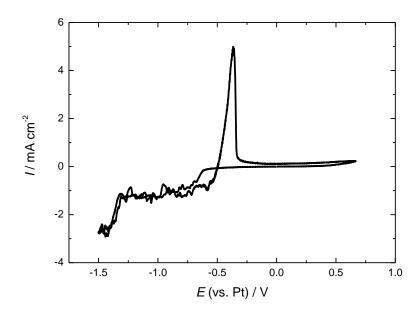
**Figure 5** Cyclic voltammetry of 2 mM [PPh<sub>4</sub>][PbCl<sub>3</sub>] + 50 mM [N<sup>n</sup>Bu<sub>4</sub>]Cl at a Pt disk electrode (surface area  $1.963 \times 10^{-3} \text{ cm}^2$ ) in scCH<sub>2</sub>F<sub>2</sub> (17.5 MPa, 360 K). The potential scan rate was 50 mV s<sup>-1</sup>.
