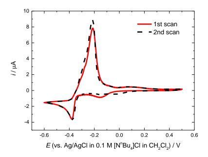
**Figure 3** Cyclic voltammograms of 0.5 mM [PPh<sub>4</sub>][PbCl<sub>3</sub>].CH<sub>3</sub>CN in CH<sub>2</sub>Cl<sub>2</sub> recorded at a 1.0 mm diameter Au disk. The supporting electrolyte used was 100 mM [PPh<sub>4</sub>]Cl and the potential scan rate was 50 mV s<sup>-1</sup>.
