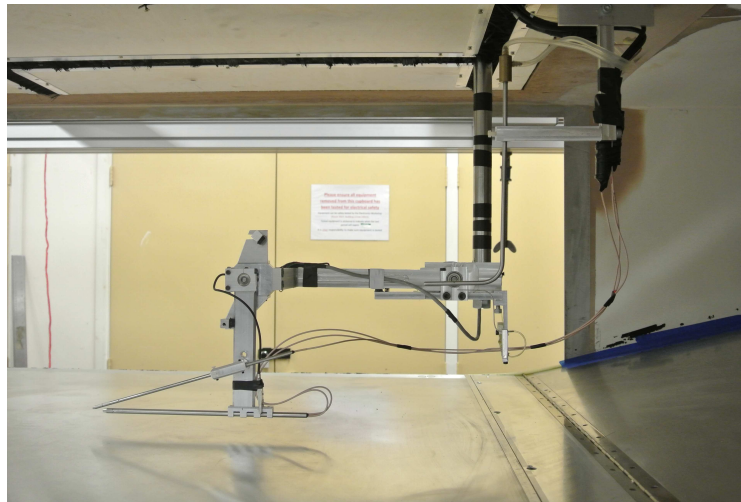
Figure A.3: Probe holders, rotating arm and traverse connection of the hot-wire system (Photo by Ronnie Hanson).
