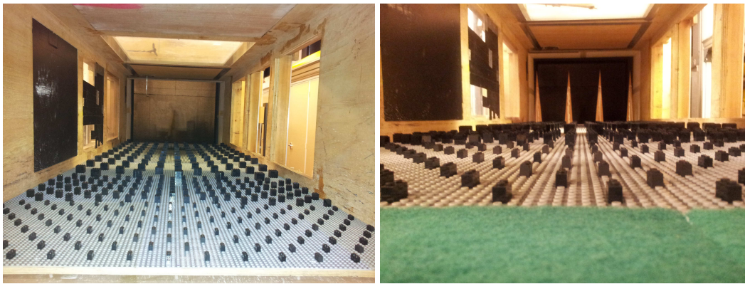
Figure 3.4: Flow conditioning setup: only roughness (left), roughness and spires (right).
