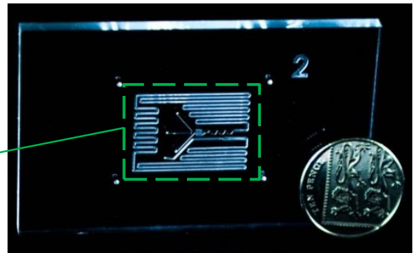
Figure 4.15 Design and fabrication of pillar induced merging chamber.
