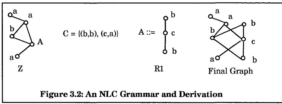
The graph language generated by GG is  $L(GG) = \{ g \in GR(\Delta) \mid Z \Rightarrow^* g \}$ , where  $GR(\Delta)$  is the set of graphs labelled with symbols from  $\Delta$ ,  $\Rightarrow$  represents a direct derivation, and  $\Rightarrow^*$  represents a derivation.
