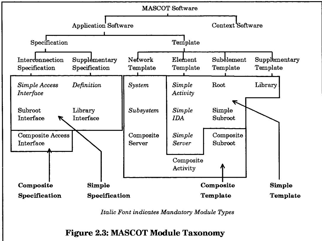
The primary structuring mechanisms used in MASCOT-3 are subsystems, composite components, and templates. Subsystems are arbitrary (well-formed) fragments of a MASCOT-3 network. Subsystems may be nested within other subsystems, thus forming a hierarchy.
