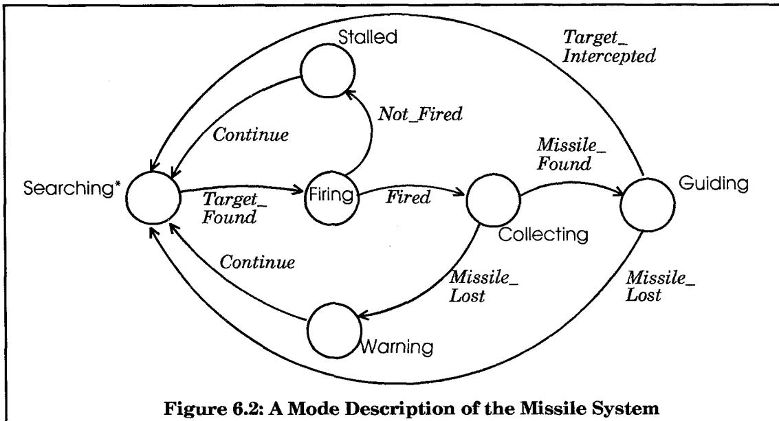
Figure 6.2: A Mode Description of the Missile System
