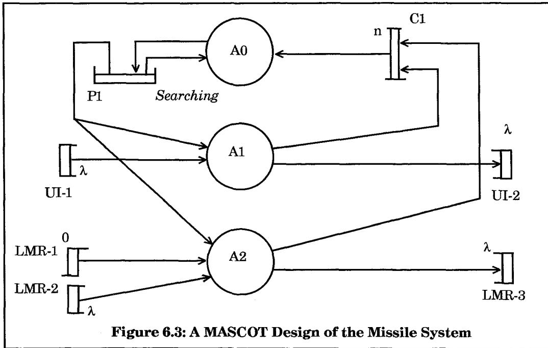
Figure 6.3: A MASCOT Design of the Missile System
