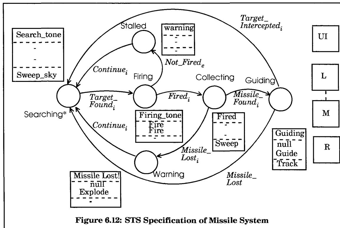
Figure 6.12: STS Specification of Missile System
