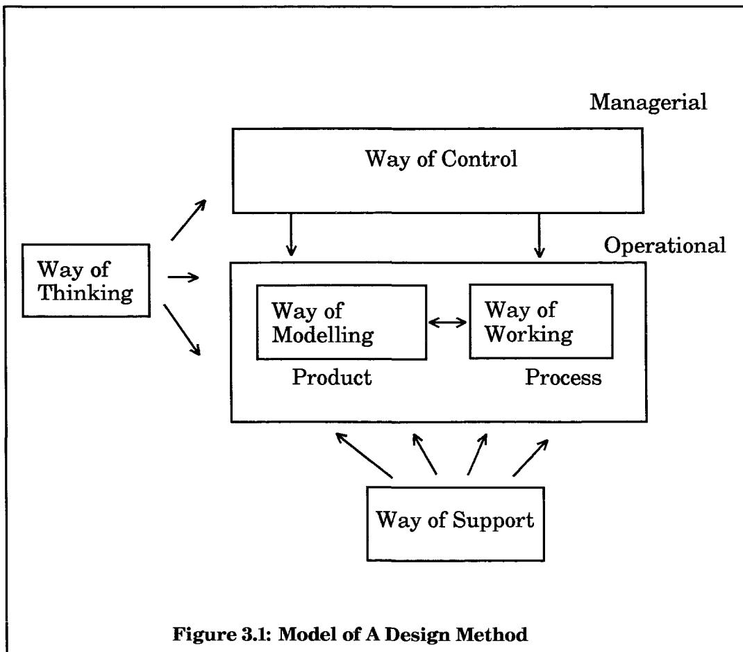
**Figure 3.1: Model of A Design Method**
