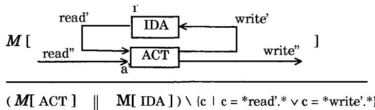
The meaning of this daughter graph, is the parallel composition of the meanings of the nodes. The actions which communicate on both read' and write' channels are hidden.
