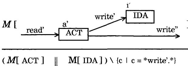
The meaning of this daughter graph, is the parallel composition of the meanings of the nodes. The actions which communicate on the internal channel are hidden.
