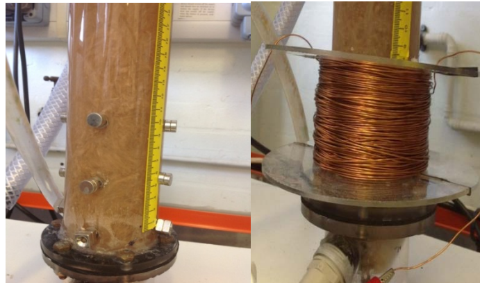
Figure 1. The installation of permanent magnet to reactor R2 and electromagnet to reactor R3.
