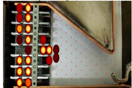
Fig. 11 events at B in Fig 9, 6.960 ms and arc voltage 283.9V. (mode 1, 3,10,20,30,40,50,60%)
