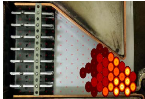
Fig. 8 The arc at the 3 ms. Imaged using mode 1 with contours at 30,40,50,60,70,80,90% of local I_{max}(t) = 339.3 .
