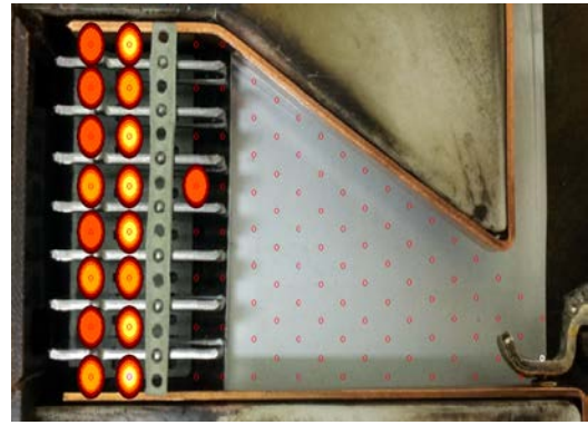
(a) At 6.047 ms with arc voltage 288.6 V.
