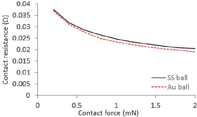
Fig. 7 Comparison of the contact resistance from the simulation and the experiments.
