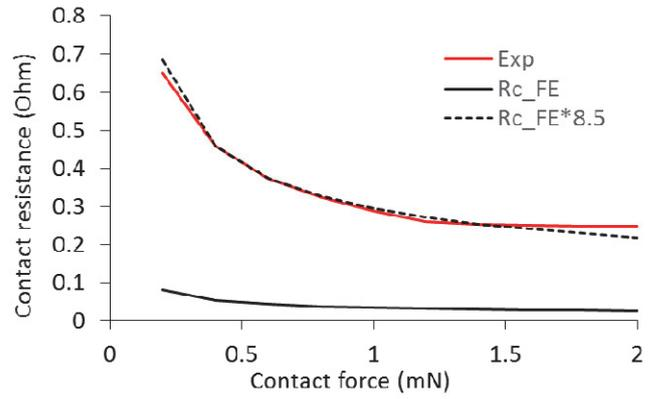
Fig. 11 Comparison of the contact resistance from the simulation and the experiments for the composite 500 nm Au/50  $\mu\text{m}$  CNT, also the simulated one with an applied factor to account for surface roughness and thin film effect.
