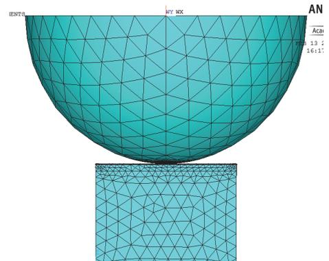
Fig. 3 Geometry of a finite element model of a 2 mm ball making contact with a Au/MWCNT substrate.
