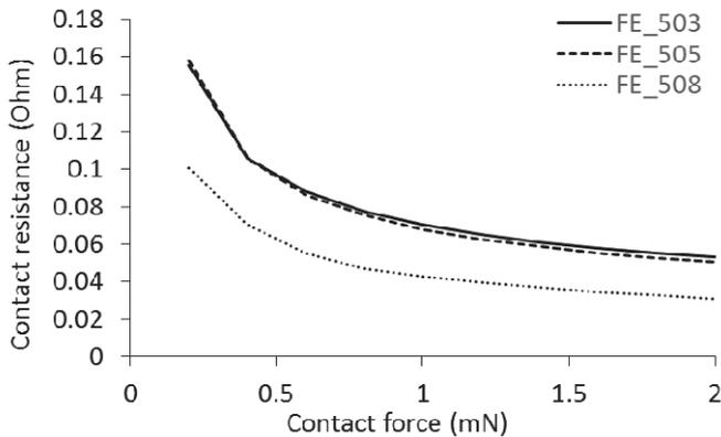
Fig. 10 Calculated contact resistance based on the FE modeling and the measured sheet resistance, for the composites with different layer configurations.
