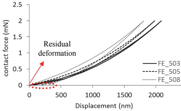
Fig. 8 Simulated force-displacement results for the samples with different layer configuration. 503, 505, 508 in the legends means 300 nm, 500 nm and 800 nm gold coated on 50  $\mu\text{m}$  CNT.
