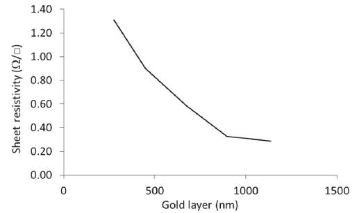
Fig. 5 Sheet resistance as a function of the thickness of nominal sputtering gold layer, the gold is coated on  $50 \mu\text{m}$  CNTs.
