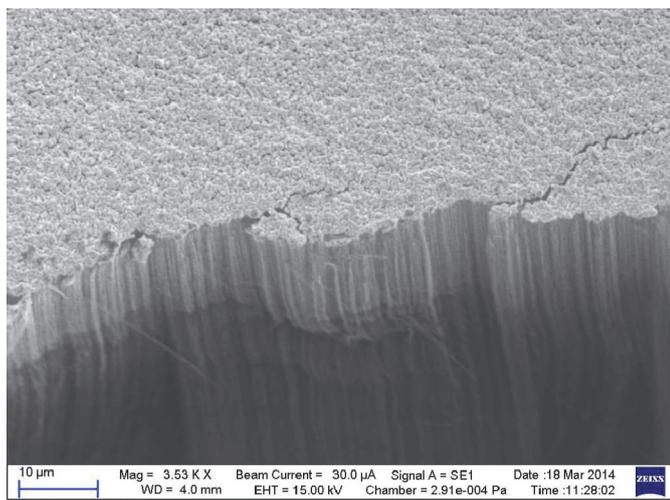
Fig. 2 SEM images of a 500nm Au/50  $\mu\text{m}$  CNT composite, showing the penetration of gold into MWCNT.
