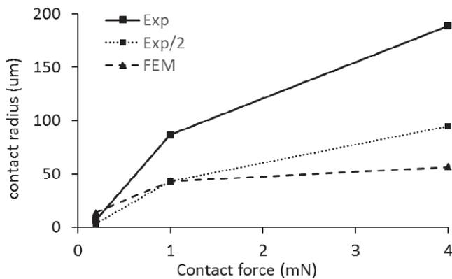
Fig. 13 The simulated contact radius for the loads 0.2 mN, 1mN and 4 mN, compared to the values from the fitting circles of the failed area in Fig. 12.
