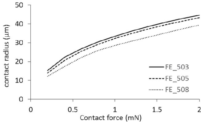
Fig. 9 Simulated force-contact radius results for the samples with different layer configuration.
