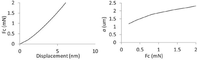
Fig. 6 Simulation results of Fc-D and  $a$ -Fc results for the Au-Au contact, the simulation is with gold solid ball, and  $a$  is the contact radius.
