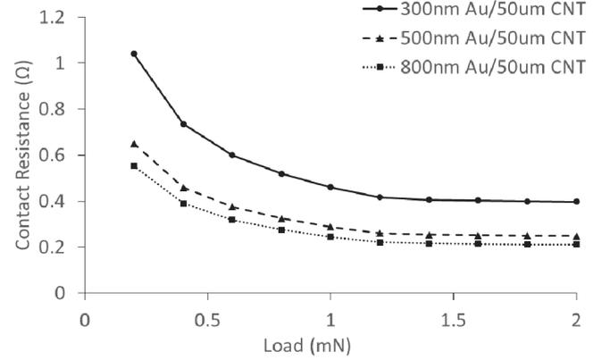
Fig. 4 Contact resistance results from nano-indentation tests as a function of contact forces, for the composites with different layer configurations.
