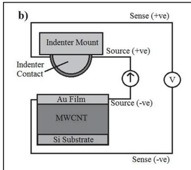
Fig. 1 Four-wire measurement system integrated into the nano-indentation, to measure the contact resistances. The current source and contact voltage drop are supplied and measured by a data acquisition module. (After [7])
