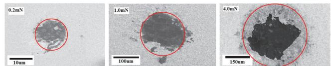
Fig. 12 SEM images of the failed sites on the 500 nm Au/50  $\mu\text{m}$  MWCNT composite for loads 0.2 mN, 1 mN and 4 mN (after [5]).
