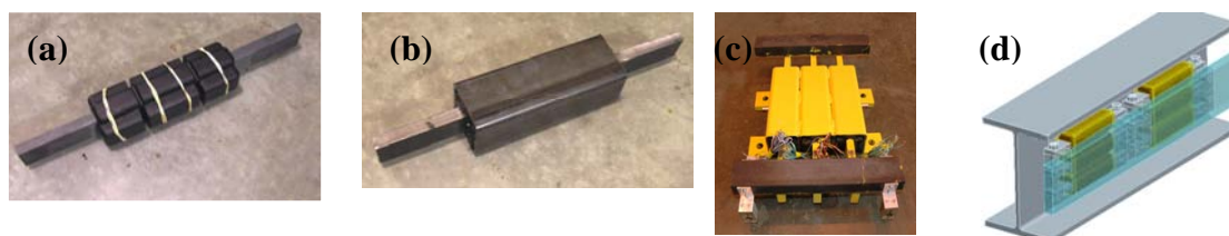
Figure 2. Fabrication of compressed elastomer damper: (a) elastomeric material wrapped around longitudinal bar; (b) elastomeric material and bar compressed into the steel tube; (c) damper bottom view with additional bolted transverse bars in place, and (d) installation to beam web
