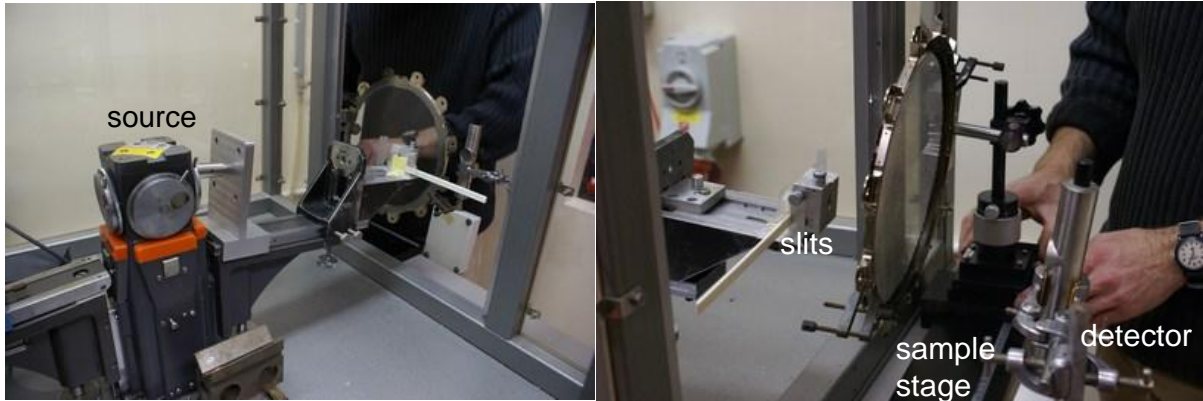
Figure 32 X-ray absorption machine with screen grid in place for measurement
