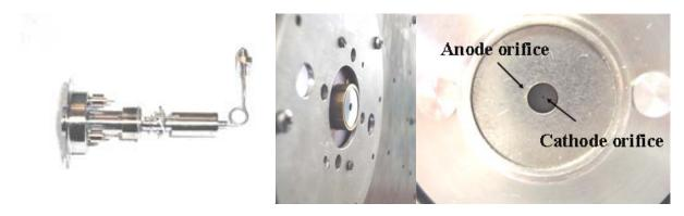
Figure 1a T5 Hollow Cathode Assembly, Figure 1b T5 mounted to UK-25 back plate, and Figure 1c T5 face
