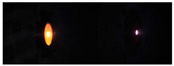
Figure 16 T5 HCT during operation with argon at 70.3W (3.2A) at 21V with 0.05mgs<sup>-1</sup> (left) and 12.8W (0.8A) at 15V with 0.8mgs<sup>-1</sup> (right)
