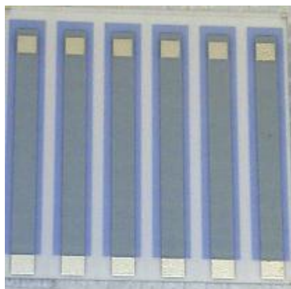
Figure 1: strips of thick film reference electrodes fabricated on a common “snapstrate” showing silver electrical connections at bottom and window exposing silver/silver chloride electrode at top
