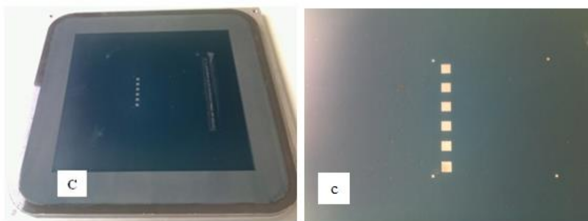
Figure 3-10: Thick-film screen (C) and mesh opening (c) for the third layer
