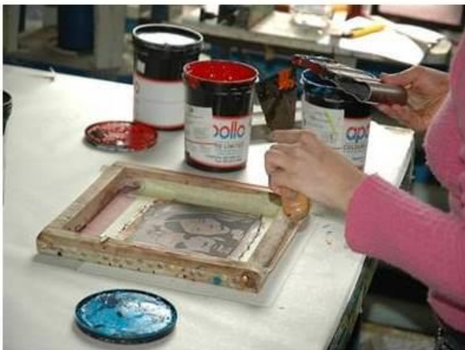
Figure 2-21: Ways of screen printing: (left) hand printing (photo: M. Karvos) and (right) mechanical printing
