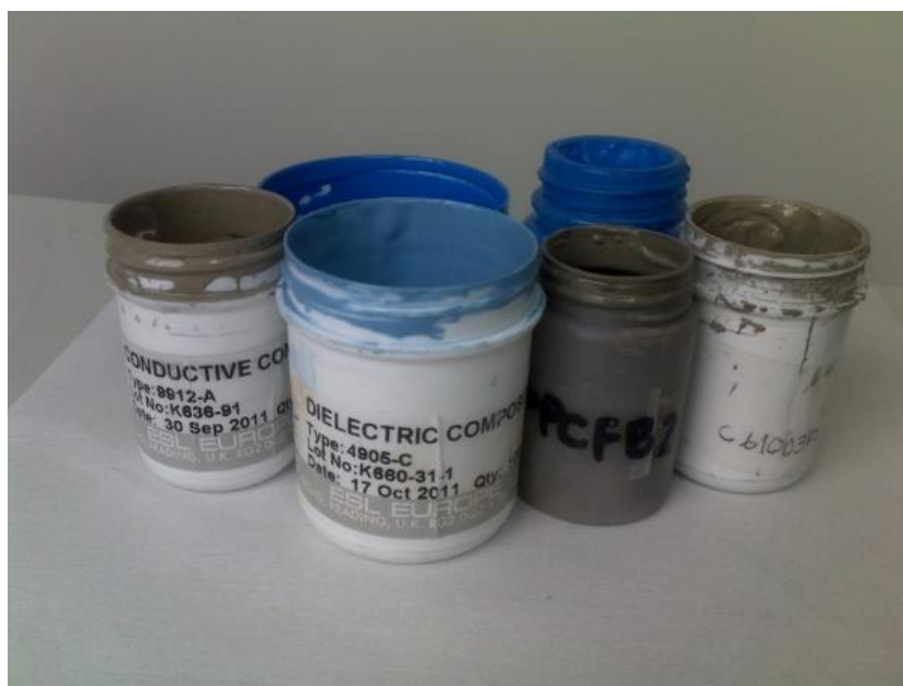
Figure 3-4: Different types of pastes used in the manufacturing process
