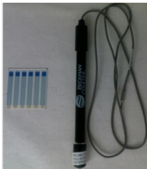
Figure 2-16: Comparison of the conventional silver-silver chloride reference electrode (right) and the thick-film screen printed (left) ones, shown on same scale
