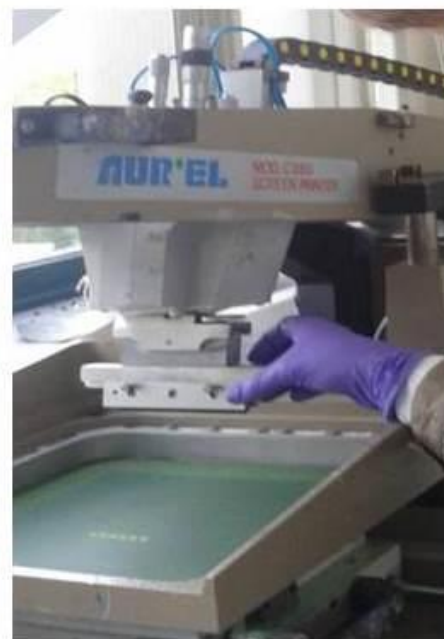
Figure 2-21: Ways of screen printing: (left) hand printing (photo: M. Karvos) and (right) mechanical printing
