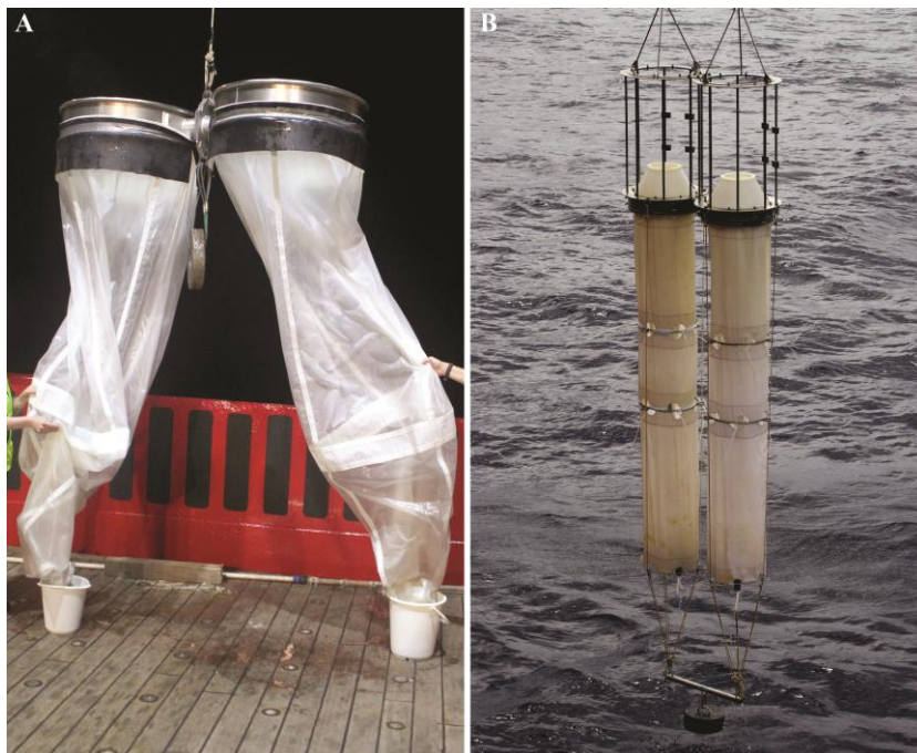
Figure 2.3 Nets used for pre-dawn zooplankton (A) and mid-day microplankton (B) sampling on AMT24 cruise.
