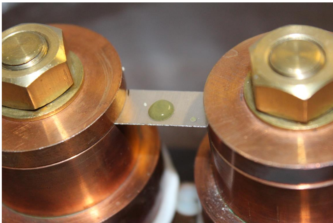
Figure D- 2: Wet sample loaded on the iridium strip between the two copper terminals.
