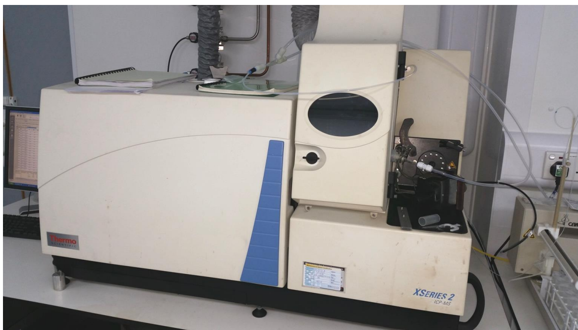
Figure A- 6: The X-Series II quadrupole ICPMS at The University of Southampton's Isotope Geochemistry Mass Spectrometry Facility
