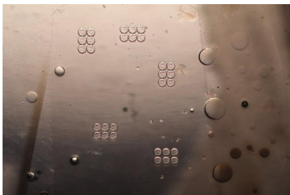
Figure 4-3: Resin mounted and laser ablated (circular pits) AC-E and SY-3 where resin interaction is possible due to vesicles and thin edges of glass beads.
