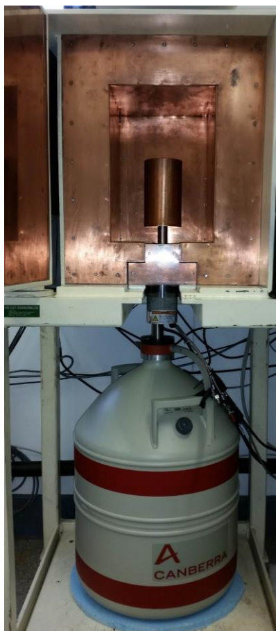
Figure A-2: One of eight Canberra HPGe detector with dewar and Cu coated Pb shielding at GAU-Radioanalytical, Southampton, UK
