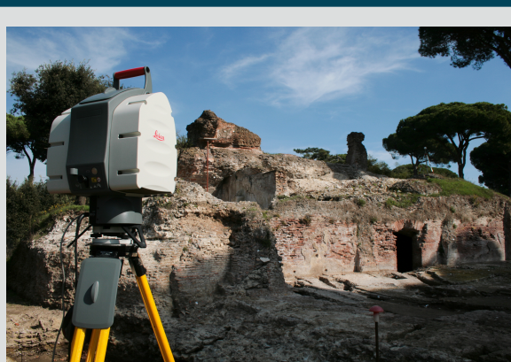
Figure 17: Laser scanning the Cistern complex at Portus using a Leica ScanStation
