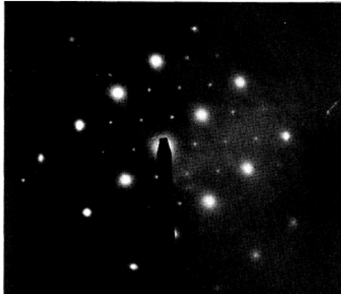
Figure 2.24: TEM diffraction of Fe 3 Al κ 1 phase showing DO 3 structure [131]
