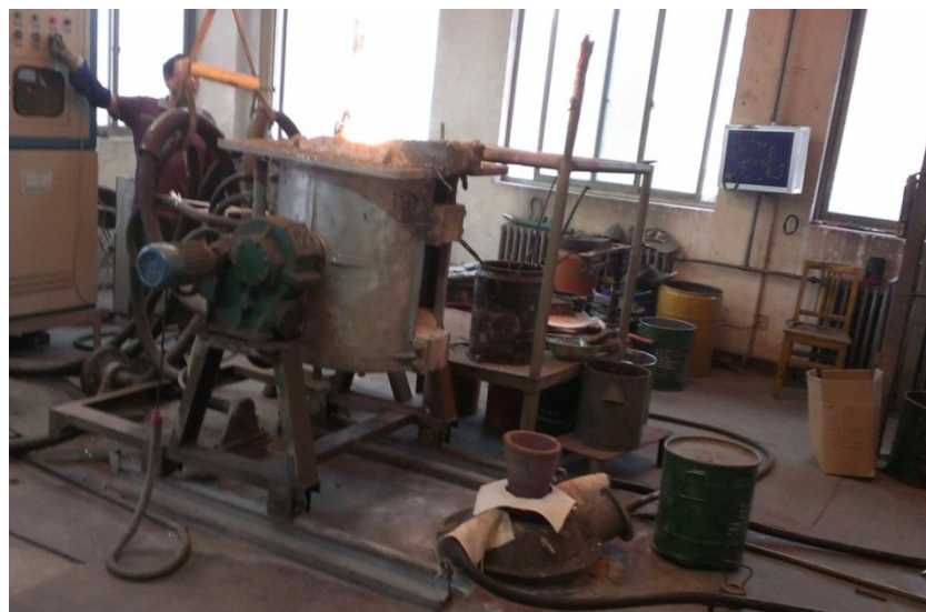
Figure 3.2: An induction furnace loaded with component metal, an atomisation chamber inlet with ceramic funnel attached
