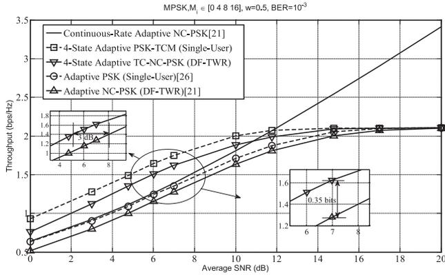
Fig. 10. Throughput of four-state adaptive TC-NC-PSK.
