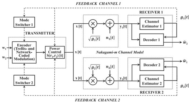
Fig. 2. System and channel models (broadcast stage).
