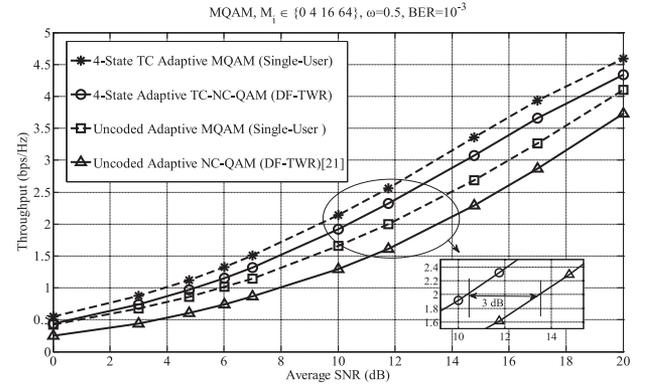
Fig. 12. Throughput of four-state adaptive TC-NC-QAM.
