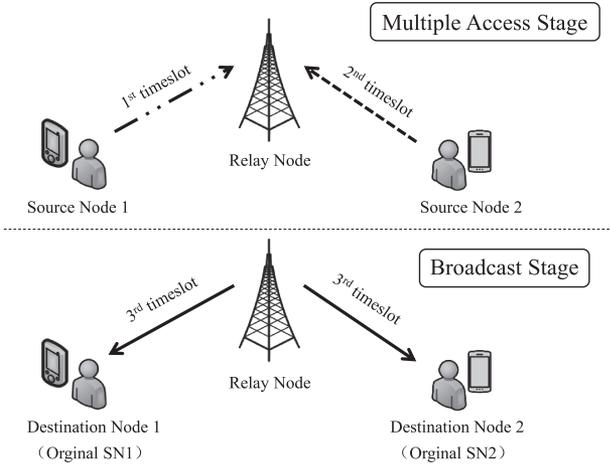
Fig. 1. Three time-slot DF-TWR.
