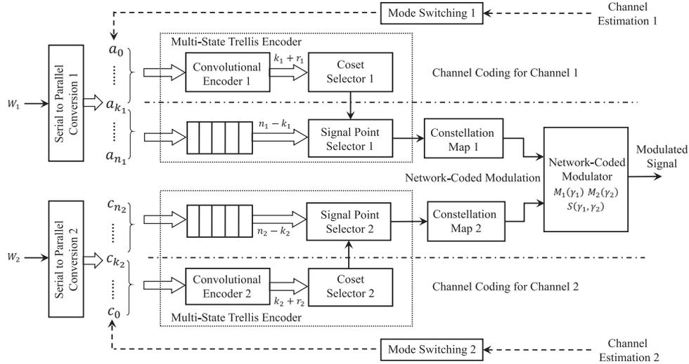
Fig. 3. Transmitter design of adaptive TC-NCM.
