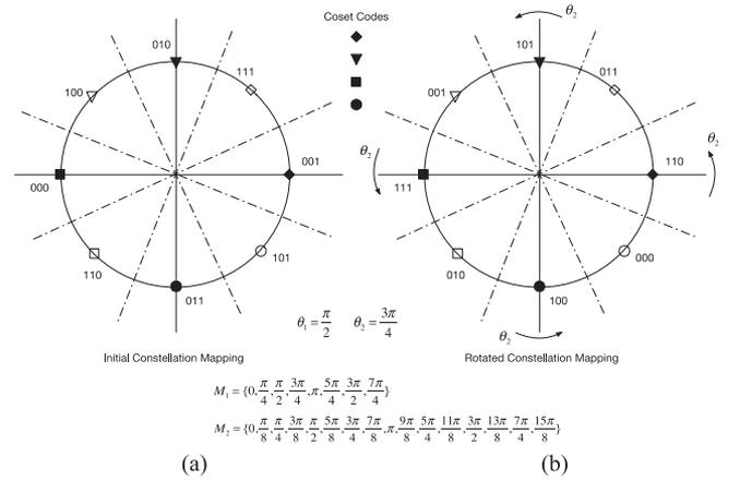
Fig. 6. Mapping rule of set-partitioning-based TC-NC-8PSK. (a) Coding design and (b) decoding design.
