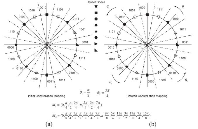
Fig. 5. Mapping rule of set-partitioning-based TC-NC-16PSK. (a) Coding design and (b) decoding design.
