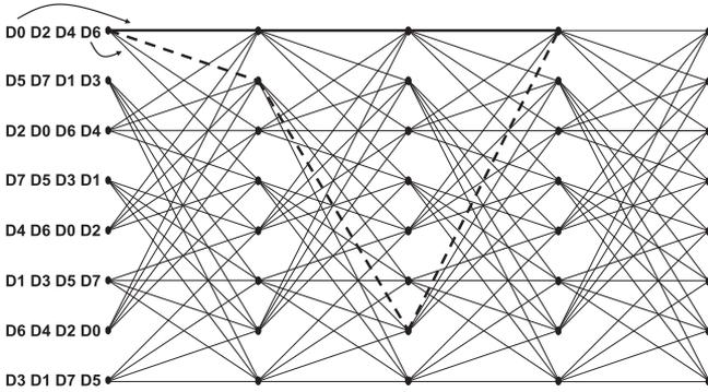
Fig. 7. One possible error path in TC-NC-16PSK (eight-state trellis).
