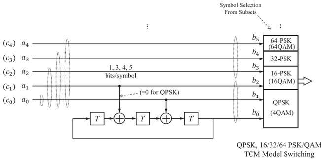
Fig. 4. Structure of the multirate trellis-based convolutional encoder (eight-state QPSK(QAM)/16PSK(16QAM)/32PSK/64PSK(64QAM)-TCM).
