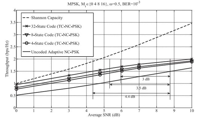
Fig. 11. Throughput versus average SNR for different number of states in TC-NC-PSK.
