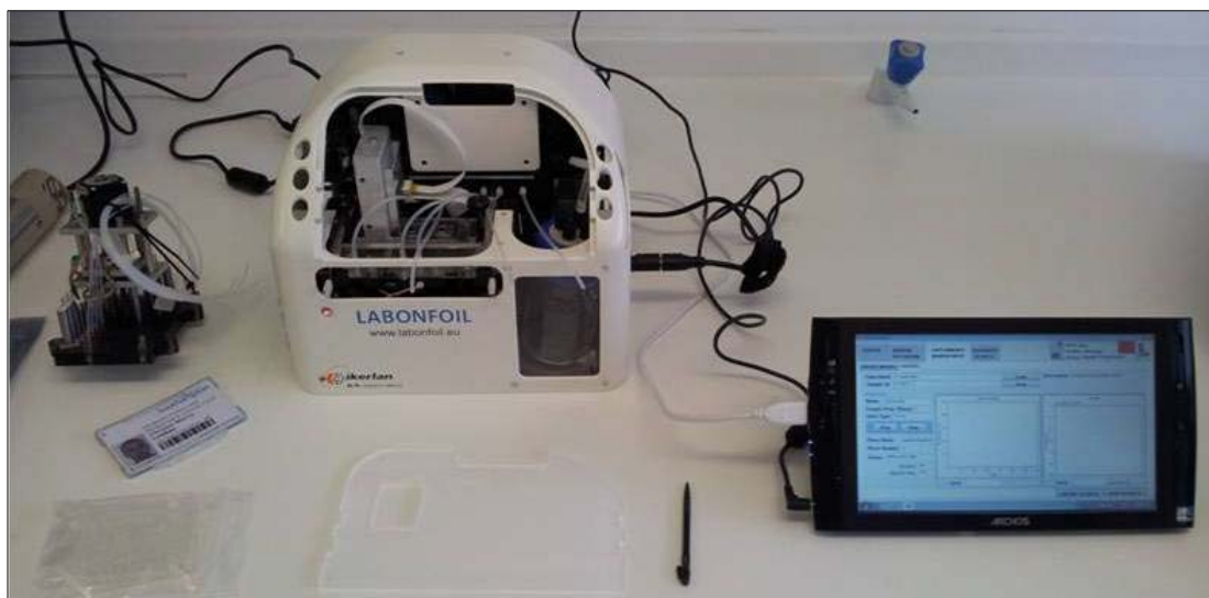
Figure 14 Image depicting the LabCardReader, a lab-on-a-chip system developed as part of the European LABONFOIL project. The device is plugged to a power source and connected to a tablet PC running the associated software.
