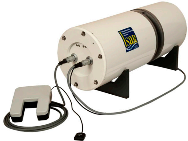
FIG. 1. External view of the ISAR instrument showing the shutter open. The optical rain sensor and the GPS antenna are in front of the instrument.
