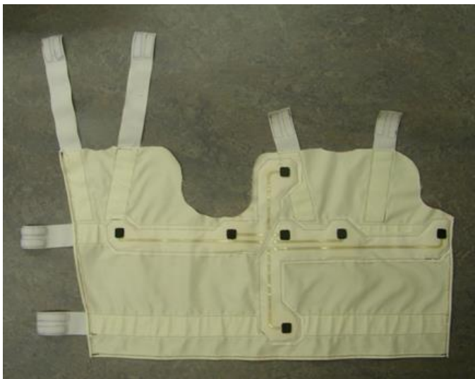
Fig. 7. The Frank configuration vest with the screen and stencil printed patches and elastic strips attached.
