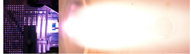
Figure 5: Inductive discharge (generator and jet), nitrogen
