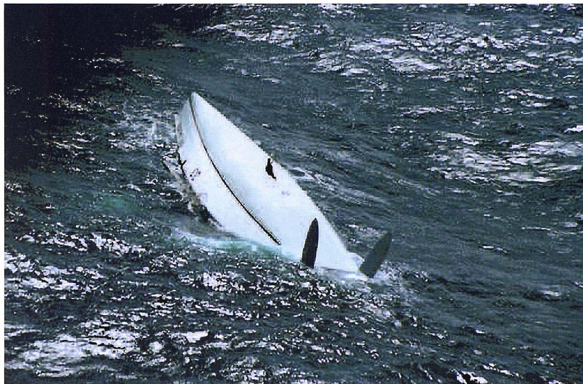
Figure 6.1: The upturned hull of “Exide Challenger” lying in the Indian Ocean after her keel fin broke. Skipper Tony Bullimore had to be rescued by a ship of the Australian navy and the yacht was abandoned. Photo credit: Guy Magowan/PPL.
