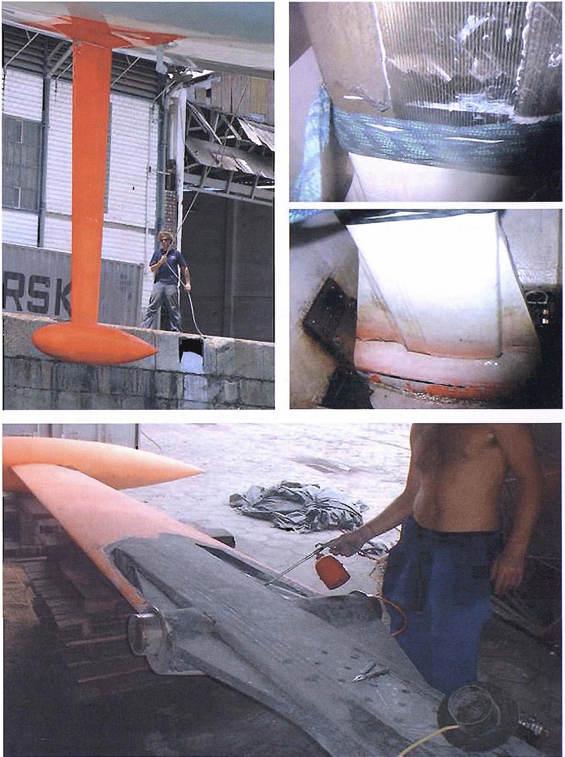
Figure 6.3: Damage suffered by the keel of “Bobst Armor Lux” during Leg 4 of the 2002-03 Around Alone Race. Top right: cracked fibres on the keel beam above the pivot axis. Middle right: wide crack between the pivot axis fairing and the keel beam. Bottom: the keel structure exposed for inspection.
