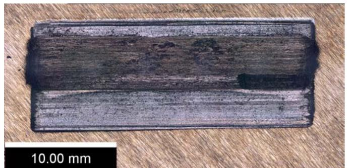
Figure 12 Optical image of the cast iron wear scar from experiment 2
