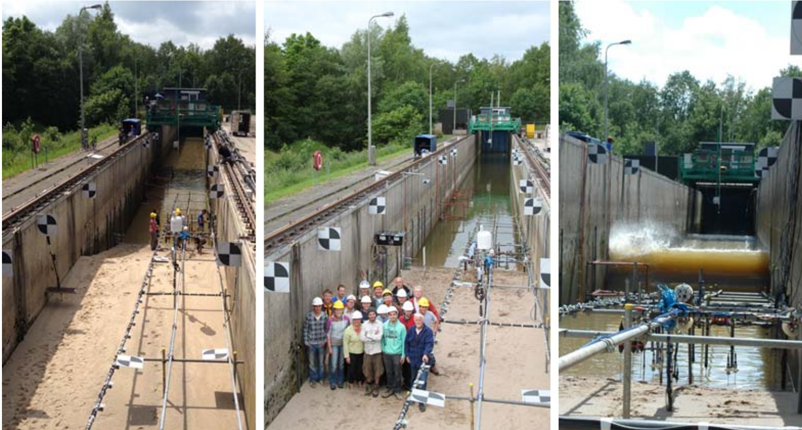
Figure 5.3 Some photos from the experiment, showing: (a) barrier setup at the start of the experiment; with the swash/over wash rig present, and bed profiling trolley (green) visible; (b) first week team photo (for scale); (c) a plunging wave breaking over the nearshore bar, followed by a shoaling wave at the location of the nearshore instrumented rig.
