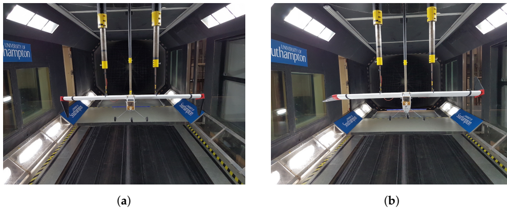
Figure 15. An example of static deflection cases. (a) Symmetric deflection; (b) asymmetric deflection.
