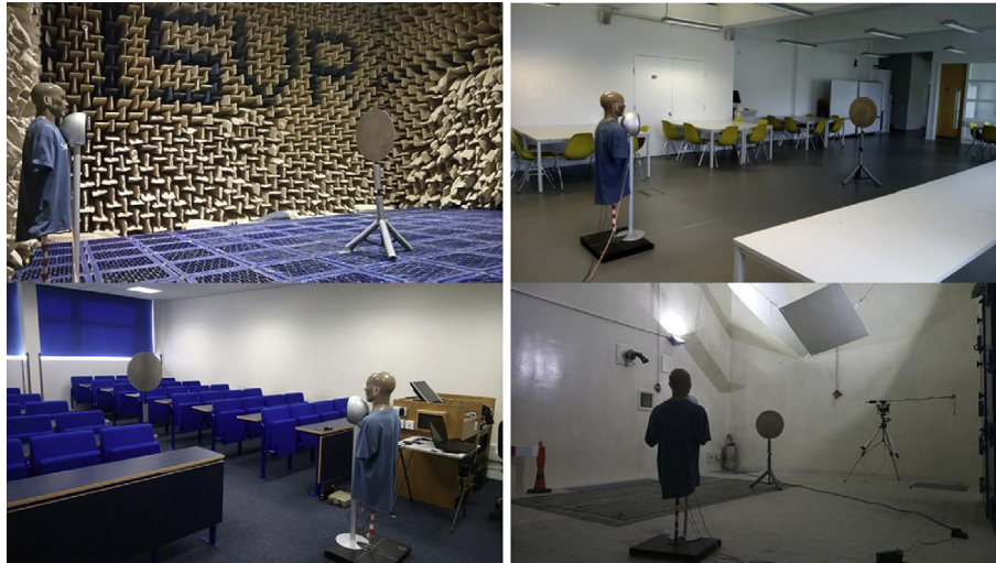
Fig. 11. The rooms used for recording the impulse responses. Top left: Room 1 (anechoic chamber, as in Fig. 1) with mid-frequency reverberation time ( RT_{0.5-1 \text{ kHz}} ) of 0.04 s. Top right: Room 2 with RT_{0.5-1 \text{ kHz}} of 0.45 s. Bottom left: Room 3 with RT_{0.5-1 \text{ kHz}} of 2.00 s. Bottom right: Room 4 (reverberation chamber) with RT_{0.5-1 \text{ kHz}} of 7.63 s. Those reverberation times (RTs) are based on impulse responses measured in the rooms (BS EN ISO 3382-1:2009, 2009) analysed using the Schroeder integral (Schroeder, 1965).
