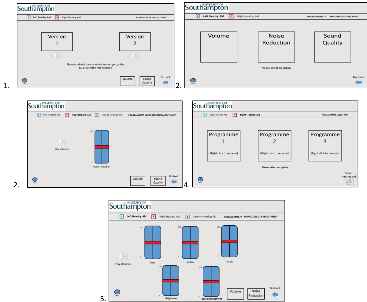
Figure 2: Screenshots from the two UIs designed for this research: (1), adjustment selection screen (used to select choice of control parameters) used across both fader and A-B selection versions; (2), A-B selection method with stimuli presentation buttons; (3) noise reduction fader from fader UI; (4), programme selection screen used on both UI versions; (5), bass, middle, treble, bass enhancement and brightness fader controls.
