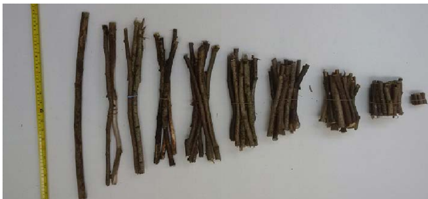
Figure 3. One particular set of 100 sticks used in the experiments with non-uniform debris.
