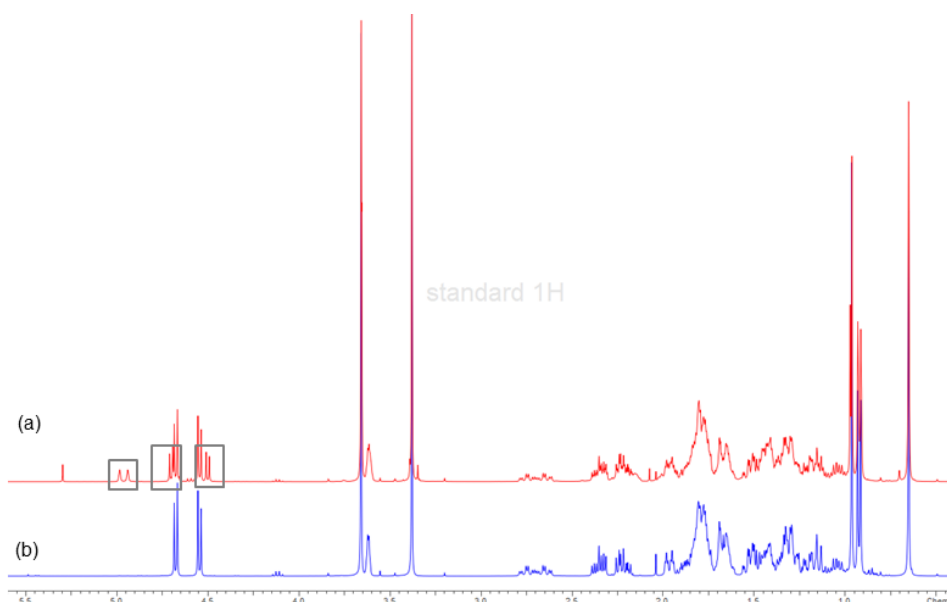
Figure 2.11 – ^1\text{H} NMR spectrum of 2.38 compound (a) before and (b) after epoxidation.
