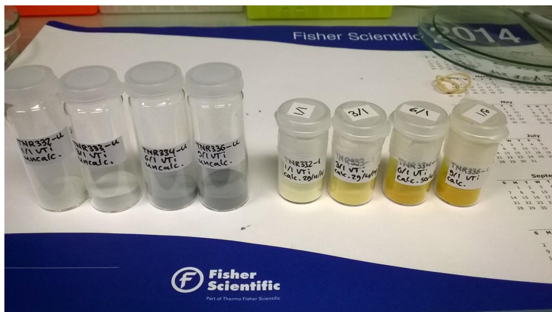
Figure 45: As-synthesised (left) and calcined (right) VTi AlPO-5 with a fixed 1% Ti and a varying loading of vanadium; from left to right: 1%, 3%, 6%, 7.5%, 9%.
