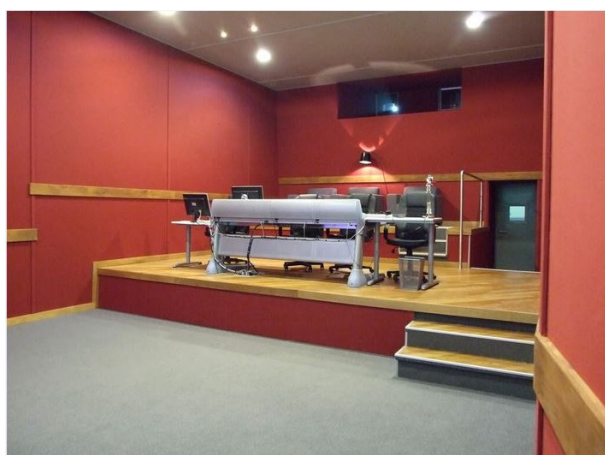
Figure 3: The rear of the room prior to testing. Wall and ceiling surfaces are absorbent down to low frequencies
