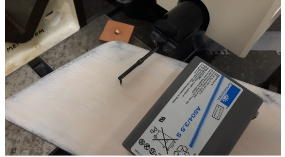
Fig. 8. Measuring the surface roughness of the foil - the black stylus is dragged across the surface of the foil and its displacement is recorded.
