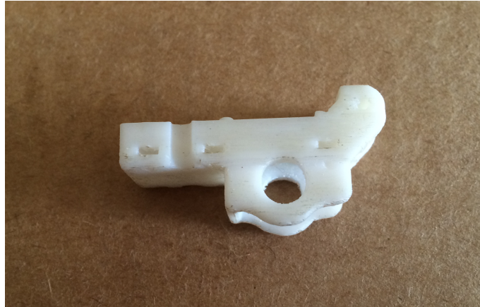
FIGURE 4.5: MCP Printed Using Fused Deposition Modelling Printer
