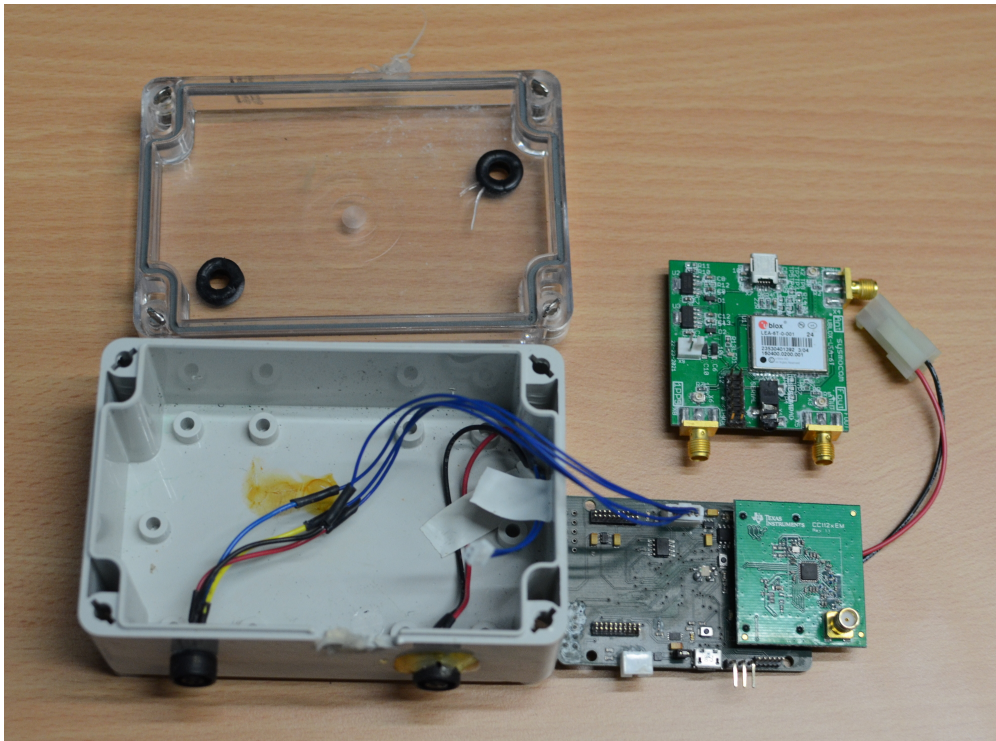
Figure 3.2: Photograph of recovered parts of a 2013 Seismic Surface Node (SSN) with DGPS module. Upper right is a Osmocom LEA-6T GPS module breakout board, lower right is a 2013 SSN board.
