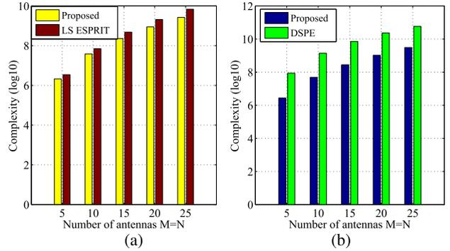
FIGURE 3. Comparison of complexity: (a) for estimating the central DOAs by the LS-ESPRIT and the proposed estimator, and (b) for estimating the central DOAs and angular spreads by the DSPE and the proposed estimator.
