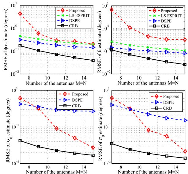
FIGURE 4. Comparison of the RMSEs as the functions of the number of BS antennas, given the SNR of 10 dB. The top two plots are the RMSEs of the three estimators for the central azimuth and elevation DOAs, and the bottom two plots are the RMSEs of the two estimators for the azimuth and elevation angular spreads.
