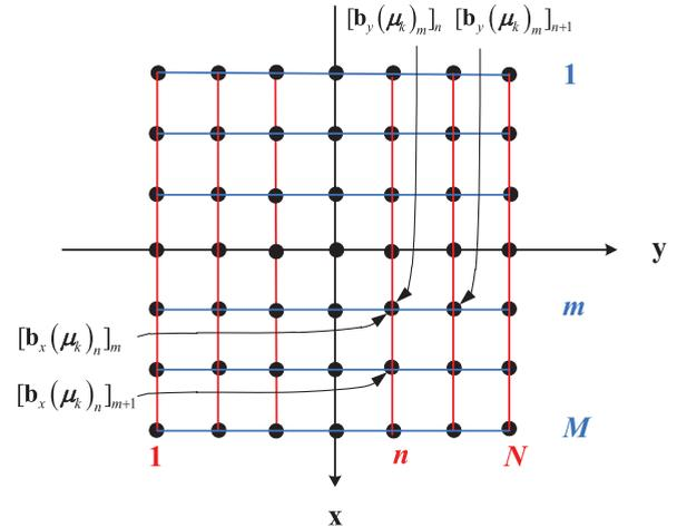
FIGURE 2. Illustration of the azimuth and elevation subarrays of URA.
