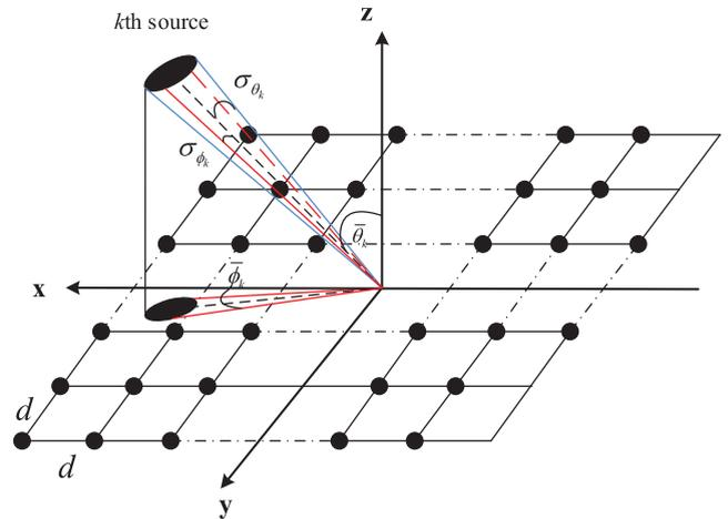
FIGURE 1. Illustration of a coherently distributed source impinging on a URA.
