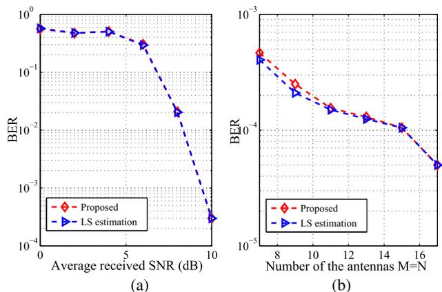
**FIGURE 7.** Comparison of the data detection performance of the two estimation methods: (a) varying the received SNR with the number of BS antennas fixed to  $M \times N = 15 \times 15$ , and (b) varying the number of BS antennas with the received SNR fixed to 10 dB.
