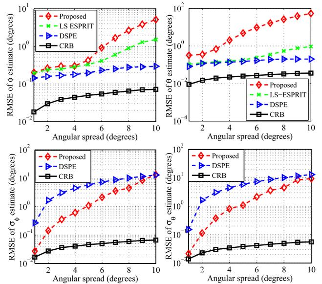
**FIGURE 6.** Comparison of the RMSEs as the functions of the angular spread  $\sigma$ , given a number of BS antennas  $M \times N = 15 \times 15$  and SNR = 10 dB. The top two plots are the RMSEs of the three estimators for the central azimuth and elevation DOAs, while the bottom two plots are the RMSEs of the two estimators for the azimuth and elevation angular spreads.
