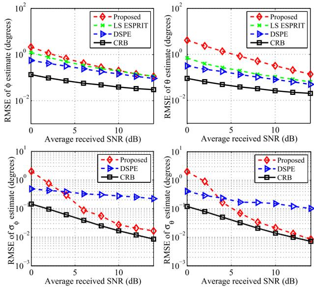
**FIGURE 5.** Comparison of the RMSEs as the functions of the SNR, given the number of BS antennas  $M \times N = 15 \times 15$ . The top two plots are the RMSEs of the three estimators for the central azimuth and elevation DOAs, while the bottom two plots are the RMSEs of the two estimators for the azimuth and elevation angular spreads.
