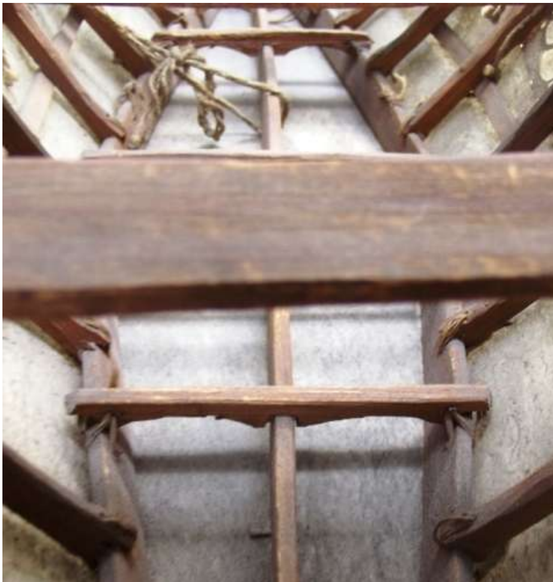
Fig.7.30. Detail of the bottom of umiak model CMH IV-X-836, Labrador, circa 1900. Note how cross-pieces are grooved to fit over the keel. Photo by E. Anichtchenko.
