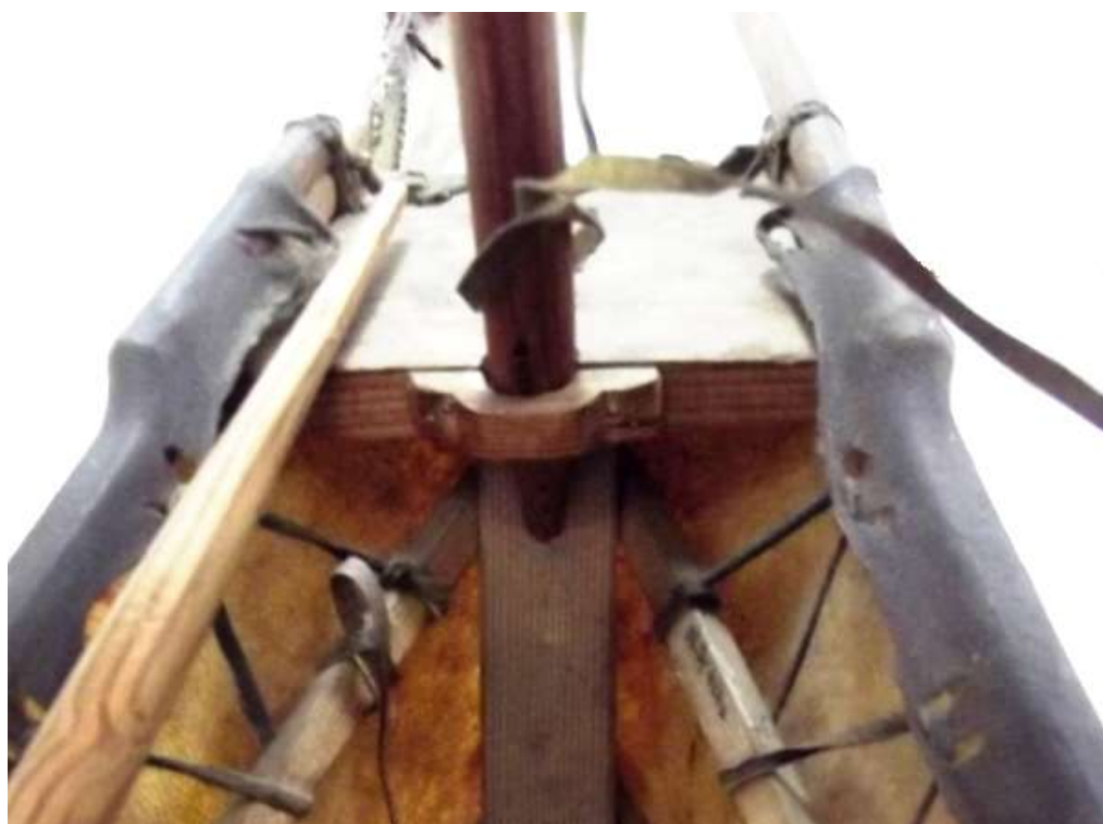
Fig.7.29. Mast brace, umiak model CMH IV-A-424, west coast of Greenland, circa 1961. Photo by E. Anichtchenko
