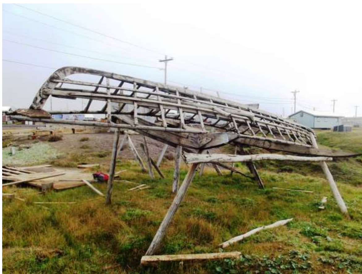
Figure 4.8. Beverly Aveoganna's umiak, Wainwright, Alaska, 2012. Photo by E. Anichchenko. Note the use of sled runners in construction of boat rack..
