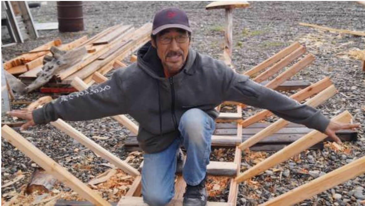
Fig.5.8. Henry Koonook demonstrates anthropometric principle behind umiak's beam dimensions. Point Hope, 2013, photo by Sarah Belcher.
