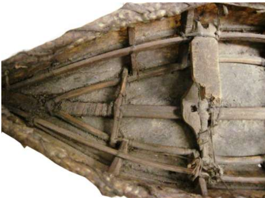
Fig.6.43. Chukchi umiak model with mast step, Anadyr region, 1904-1907. REM 2083-66. Photo by E. Anichtchenko
