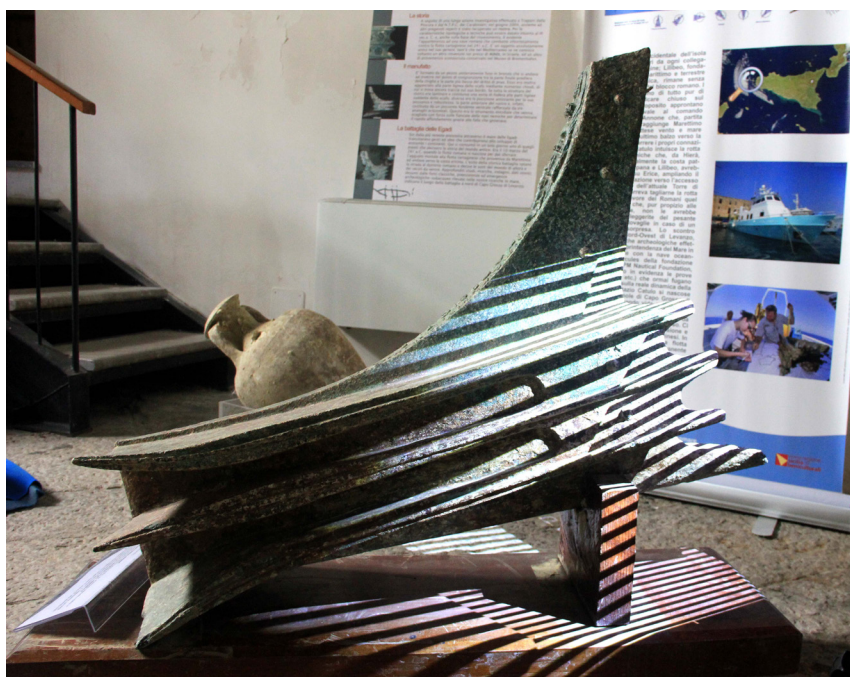
FIGURE A4.1. A STRUCTURED LIGHT SCAN IN PROGRESS ON THE EGADI 5 RAM (AUTHOR).
