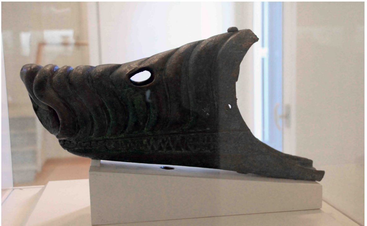
FIGURE A3.10. THE KANELLOPOULOS RAM, WHOSE DESIGN SUITS COVERING A KEEL AND STEM, A DIFFERENT DESIGN FROM THE ACTIUM PROEMBOLION (FIGURE 4.12), WHICH IS DESIGNED TO COVER THE WALES (AUTHOR).
