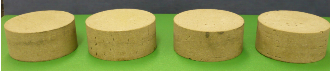
Figure 5.5: Acid leached, blank, synthetic silica-cemented sandstone sample (far left) and corresponding synthetic samples with aligned penny-shaped voids ( 90^\circ , 45^\circ and 0^\circ respectively from left to right). The samples were cored along the grain layering which is in the same plane as the penny-shaped voids. Sample diameters are 50 mm.
