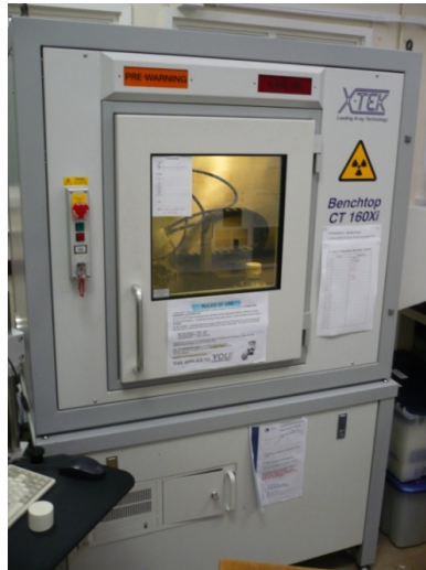
Figure 4.6: X-TEK Benchtop CT 160Xi scanner with sample inside.
