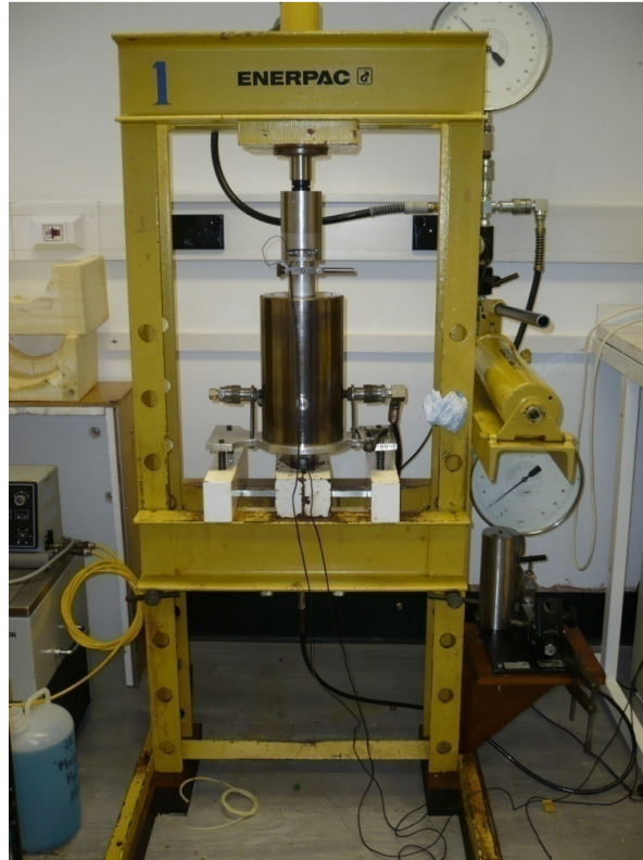
Figure 4.2: The ultrasonic pulse-echo system when installed inside the Hoek high pressure cell and steel load frame.
