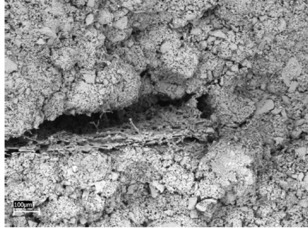
Figure 4.9: SEM image example showing grain size variation and material within the penny shaped void. Note scale bar is 100 \mu\text{m} in the bottom left hand corner.
