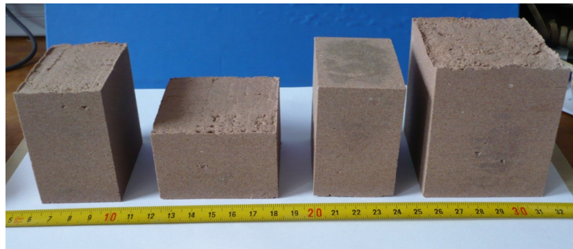
Figure 5.3: Blocks after drying and heating in furnace.
