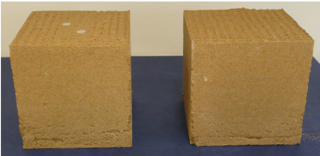
Figure 6.4: Blocks after drying and heating in the furnace. Aluminium discs on the top of the left block only act as a reminder to it being the fractured block.
