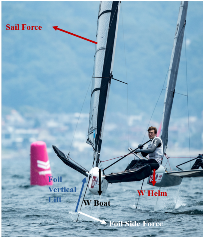
Figure 1: Forces acting on an International Moth whilst sailing.
