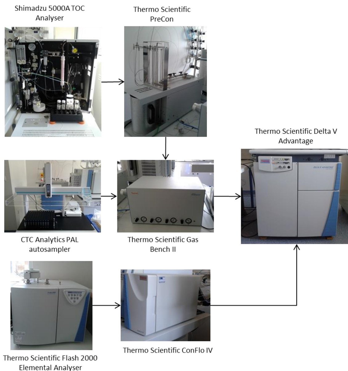
Figure 4-3. Instruments used to perform stable isotope analysis of dissolved and particulate organic and inorganic carbon for the samples collected during the mesocosm campaigns in Sweden (2013) and Norway (2015).
