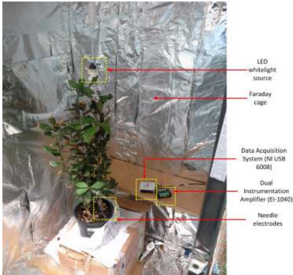
Figure 3.11: Experimental setup (followed in Rome/Florence) to obtain electrical response from a Bay leaf plant when exposed to white-light
