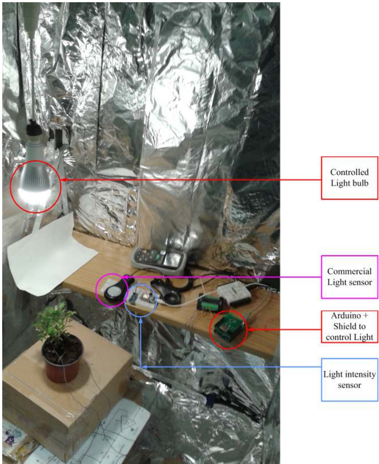
Figure 3.26: New experimental setup to collect data by controlling light pulses using an Arduino
