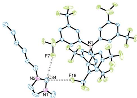
Figure 3: ORTEP representation of [HMIM][BAR f ]. Thermal ellipsoids are drawn at 50% probability and hydrogen atoms are omitted for clarity. The dashed lines represent the bifurcated hydrogen bonding through the C2 position (labelled C34) of the imidazolium ring.
