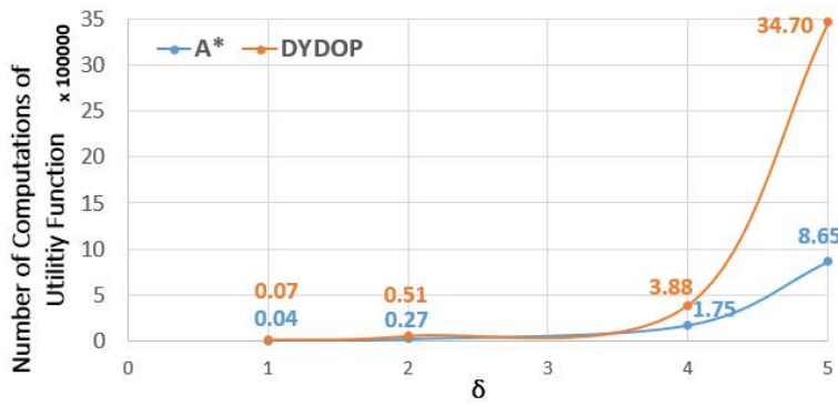
FIGURE 6.8: The Number of Utility Computations Required to Solve the Optimal Dispatch Problem Using A*-based approach and DYDOP
