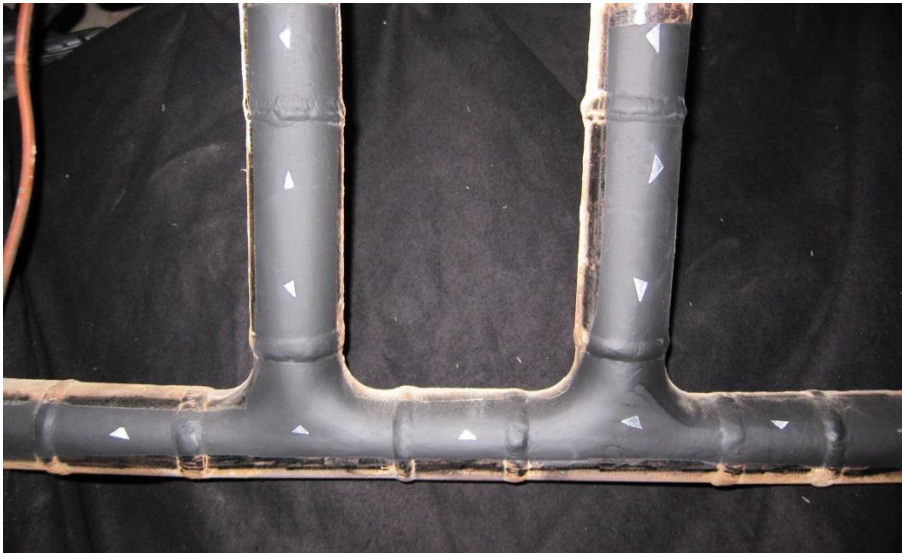
Figure 7-16 – Site two prepared with coating of matt black paint. Motion compensation markers stuck on either side of every weld to be investigated.
