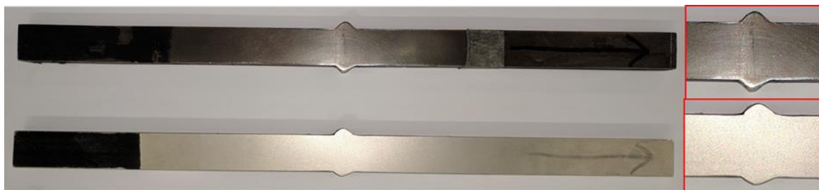
Figure 5-18 – A photo of both MU-A (top) and the physical reference specimen (bottom). The weld geometries of both have been enlarged in the red boxes to the right.
