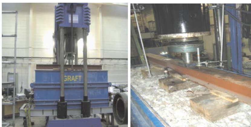
Figure 2-10 Geopavement and railway accelerated fatigue testing facility at Heriot-Watt University (Kennedy, et al., 2012)
